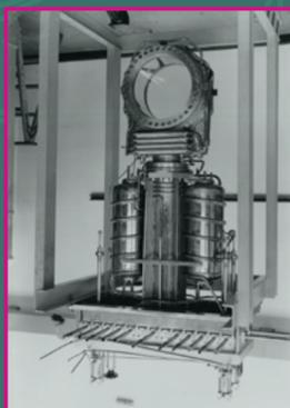
The 32 cm hydrogen chamber, the first bubble chamber built at CERN to do physics.
