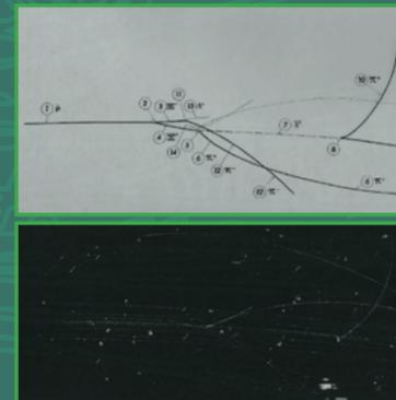
Production of an antixi particle ( $\bar{\Xi}$ ) in the 81 cm chamber.
