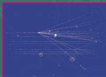
The interaction of a 24 GeV proton in the 32 cm chamber.
