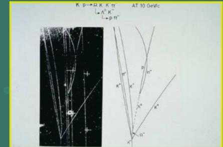
Particle tracks in the CERN 2 m liquid hydrogen bubble chamber. A negative kaon enters the chamber and interacts, giving rise to many particles, including an Omega minus.
